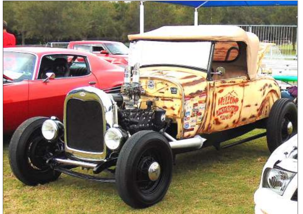
Picture of street Rod built from 30's model Ford with a flathead Ford motor
